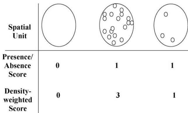
**Fig. 3.** Two methods for quantifying frequency scores. The large circles represent the spatial unit of analysis (i.e., watershed) while the small circles represent a single point stressor (e.g., mine). Presence/absence scores are based on presence of a stressor while density-weighted frequency scores are based on equal quartiles of the density of the stressor.
